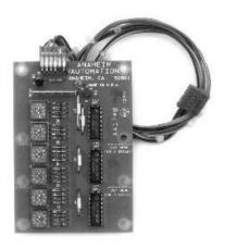
A 'CLICK POT' module consists of 10 position (0 - 9) digital pots mounted on a circuit board. One pot is used per each decade (digit). These units are available in 2, 4, or 6 decades. The user dials in the step count on the pots. Any time the motor is indexed, it will move the number of steps set on the pots. One module is required per axis. The module is connected to the indexer via a supplied 5 lead cable.
