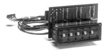
These thumbwheel switches provide an attractive way to input a step count. The user dials in the desired count on the thumbwheels, which can be mounted on an enclosure face. The module is available in 2, 3, 4, 5, or 6 decades. The module is connected via a supplied 5-lead cable.
