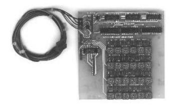
The quad board module is a 4-bank version of the clickpot module with each bank having 6 decades. The user can "dial in" 4 different move lengths and then select any one of them as needed. The module is connected to the indexer via a supplied 5-lead cable.
