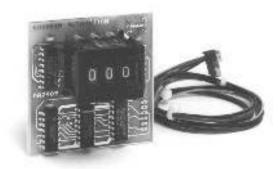
This module is similiar to the AA1760 series Thumbwheel Switch Module. It uses a "+Push and -Push" style button to increase or decrease the number on the dial. This unit also includes a single "Rotary Switch" module consisting of 10 positions (0-9), which is used as a multiplier of the Thumbwheel Switch settings.
