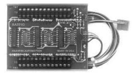
The AA2210 BCD counter interface module enables the user to select any move length from 0 to 999,999 steps using a standard PLC (programmable logic controller). Selecting the proper inputs creates a count value in steps, resulting in a move distance. The module is connected to the indexer via a supplied 5-lead cable.
